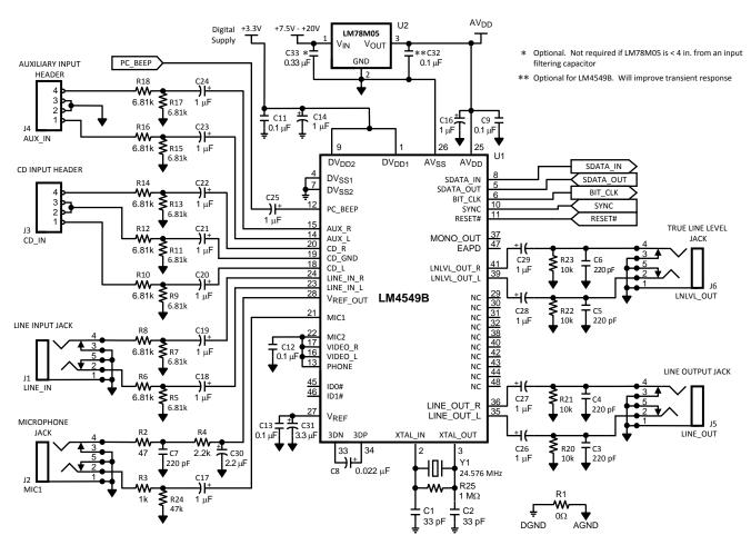
Figure 22. LM4549B Reference Design, Typical Application
