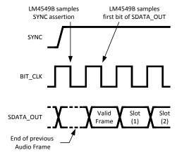
Figure 17. Start of AC Link Output Frame
