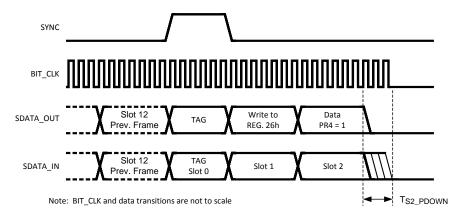
Figure 14. AC Link Power-Down Timing
