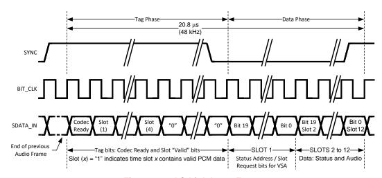
Figure 18. AC Link Input Frame
