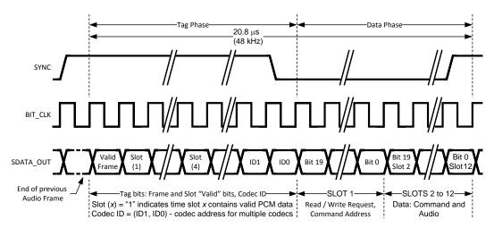
Figure 16. AC Link Output Frame
