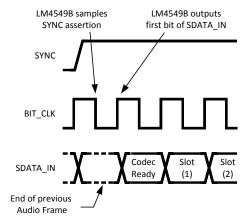
Figure 19. Start of AC Link Input Frame
