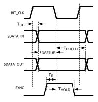
Figure 2. Data Delay, Setup and Hold
