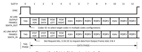
Figure 15. AC Link Bidirectional Audio Frame
