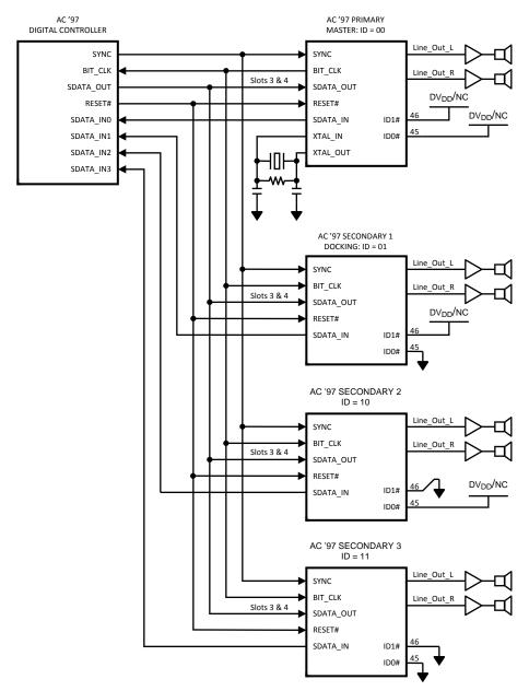
Figure 20. Multiple Codecs using Extended AC Link
